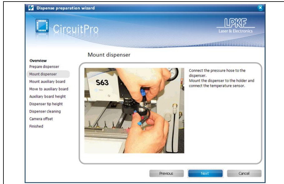
Fig. 36: Assembling the dispenser
