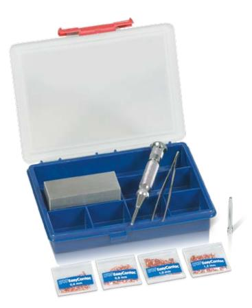
LPKF EasyContac is a manual system for through-hole plating double-sided PCBs with copper-alloy rivets. Perfect for applications where double-sided soldering is impractical. LPKF EasyContac requires no special tools or chemical baths. The portable tool set includes all the required tools. For additional information on throughhole plating refer to the TechInfo starting on page 107.
